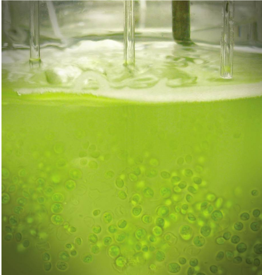
Detail of an experimental chemostat vessel with magnified ( \times 1,000 ) cells of the cultured model organism, the green alga Chlorella vulgaris . Variable sizes reflect different developmental stages, from small daughter cells to rather large mother cells. Glass tubes above the water level are used for sampling, to supply fresh medium and sterile air, and for adjusting the experimental volume. Photograph by Thomas M. Massie.
