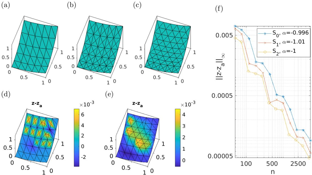
Figure 6: Example 2.7, `geomtut/parabol/cmds1.m`. Initial mesh (a), different mesh-refinements and local effects on error (b)–(e), but similar overall convergence (f).
