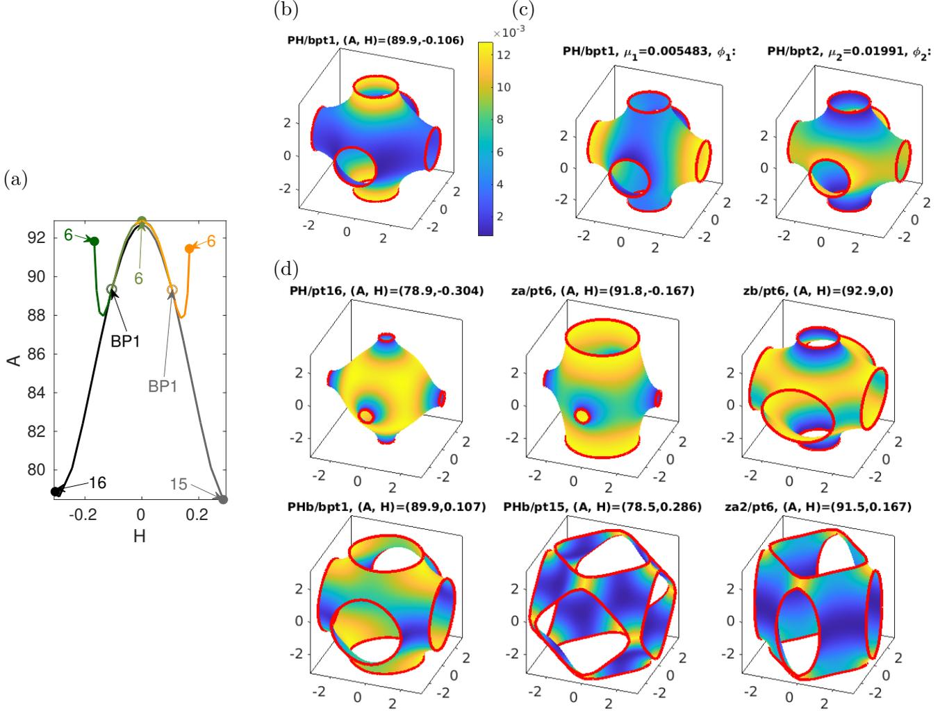
Figure 20: Some results from TPS/cmds2.m. Continuation of Schwarz P in  $H$  at fixed  $\delta = 2\pi$ . BD in (a): PH (black), PHb (grey), za (dark green) and zb (lighter green), and za2 and zb2 (orange), but altogether these are just two different branches. BP1 on PH and approximate kernel vectors in (b,c), and further samples in (d). See text for details.
