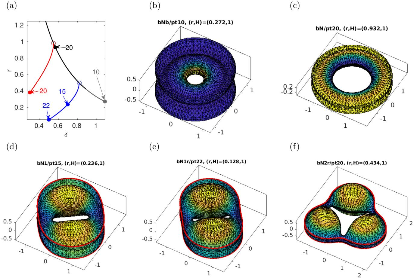
Figure 16: (a) Bifurcation diagram of nodoids parametrized by height  $\delta$ , fixed  $H = 1$ . The axisymmetric branch **bN** (black) starts near  $\delta \approx 0.88$  via (54), and in direction of decreasing  $\delta$  shows a sequence of BPs to nodoids with broken  $S^1$  symmetry, here **bN1** (blue,  $m = 2$ ) and **bN2** (red,  $m = 3$ ). Samples in (b–f), with **bN1r** and **bN2r** after some refinement.
