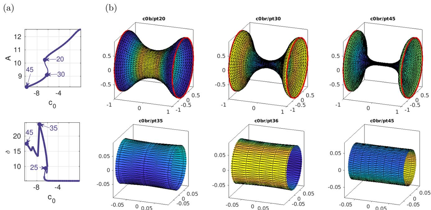
Figure 31: Results for (??) from `biocyl/cmds1.m`.  $(\alpha, \varepsilon) = (1, 1/4)$  fixed, continuation to  $c_0 < 0$ , with a bistability region near  $c_0 = -6.25$ . Initially uniform mesh of  $n_p = 1770$  points, and the 2nd plot in (a) indicates that with suitable refinement (at `pt25` and `pt35`, to  $n_p = 3561$ ) the meshes stay good. Samples in (b), with zooms of the necks to illustrate the meshes.
