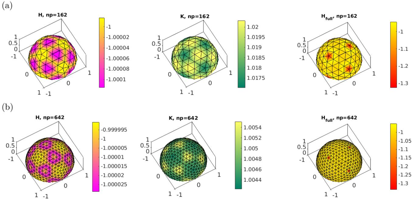
Figure 4: Discrete  $H$  (and  $K$ ) on (coarse) meshes of the unit sphere (plots cropped). Two left columns: Convergence for  $H = -\frac{1}{2}M^{-1}\langle LX, N \rangle$  and  $K = M^{-1}K$  with Voronoi  $M$ . Right column: No convergence for  $H$  (and similar for  $K$ ) at valence 5 nodes when using  $M^{\text{full}}$ .
