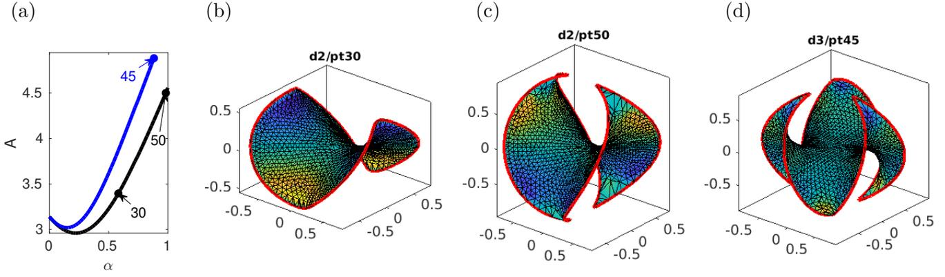
Figure 10: Results from `cmds2.m` for BCs (46) with  $k=2$  (black branch `d2`) and  $k=3$  (blue branch `d3`). Along the way in, e.g., `d2` we do 3 refinements and coarsenings, and the total number of mesh points only increases mildly from  $n_p=945$  to  $n_p=1177$ . These are really two different ( $k=1$  vs  $k=2$ ) continuation problems, out of infinitely many ( $k \in \mathbb{N}$ ), and hence the two branches in (a) are from different problems and are both stable.
