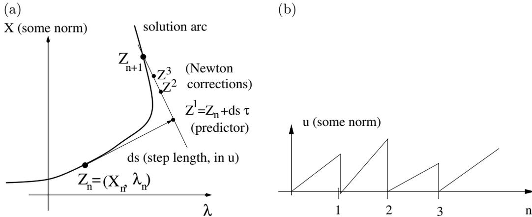
Figure 2: (a) Sketch of arclength continuation algorithm in the `Xcont` setting. (b) Illustration of the “solutions”  $u_n$ , which are only meaningful together with  $X_{n-1}$  via  $X_n = X_{n-1} + u_n N_{n-1}$ .
