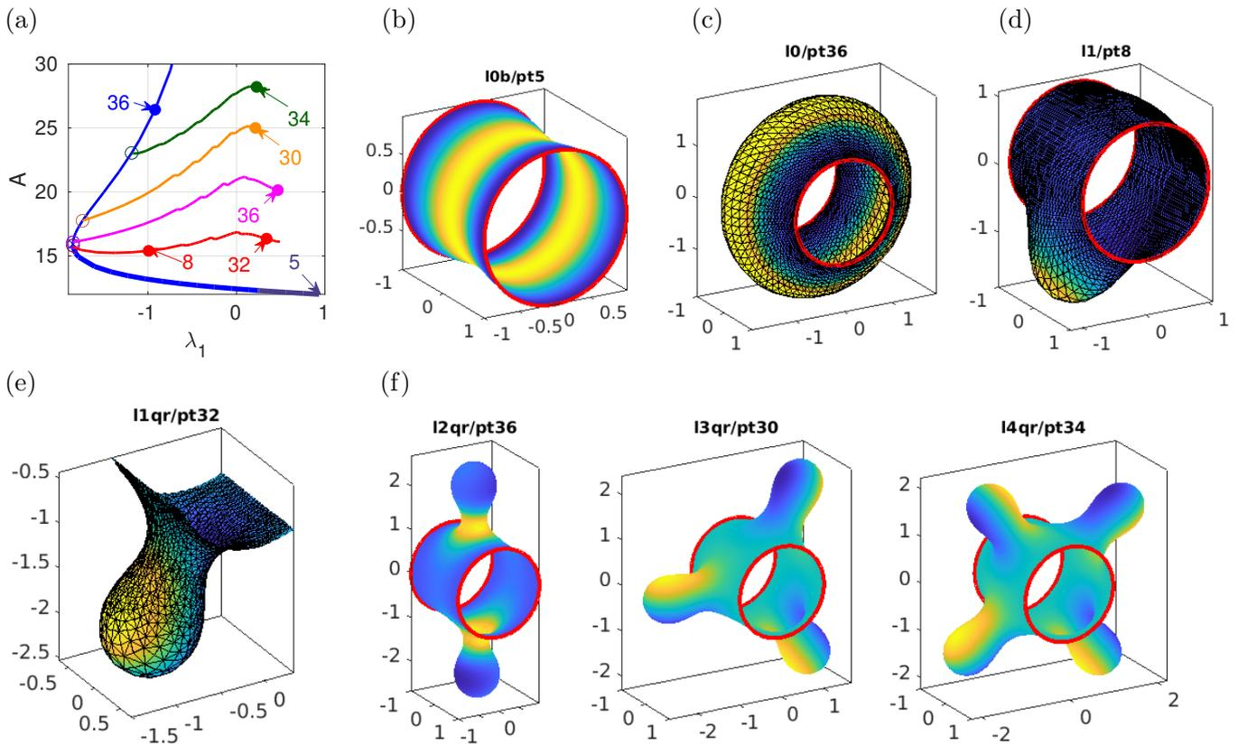
Figure 36: `cmd4.m`, continuation in  $\lambda_1$  at  $c_0 = 0.7$ . In (a): axisymmetric branch 10b (dark blue, sample in (b)), 10 (blue, sample in (c))), and four bifurcating branches, 11 (red, refined to 11qr, samples in (d) and (e), with zoom), 12 (magenta), 13 (orange), 14 (green), samples in (f). The kinks of 11–14 are due to adaptive mesh refinement every 5th step (after pt10), from  $np = 2700$  to  $np \approx 3600$  at the end of each branch.
