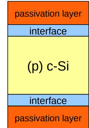
p,n-type c-Si wafer with different passivation:
