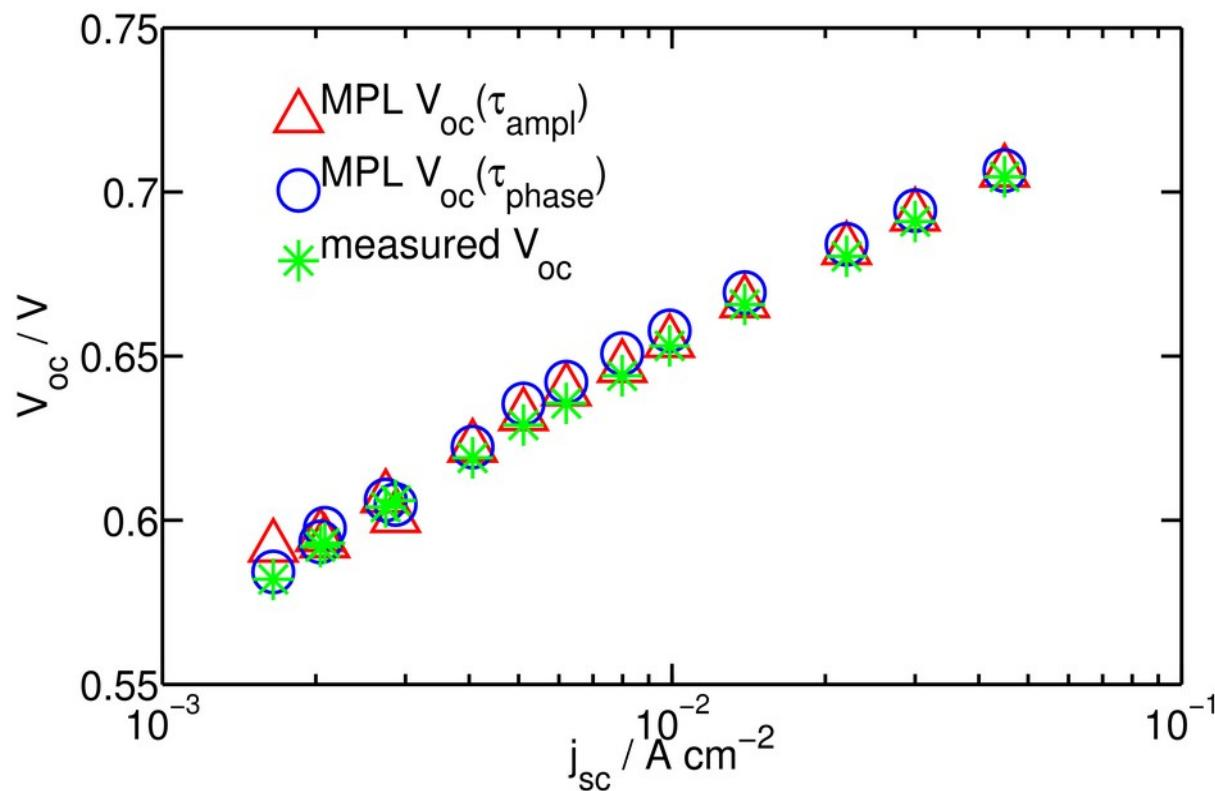
→ Good agreement between measured  $V_{oc}$  and  $V_{oc}(\tau_{\text{eff}})$  by MPL
